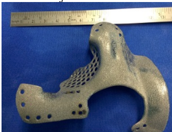
Fig. 3A. Titanium prosthesis to reconstruct the defect: mashed part - orbital floor; holes for bone fixation - frontal, nasal, zygomatic and right maxilla.
